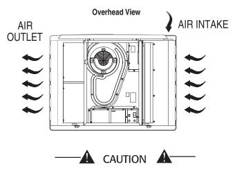
The maximum ambient temperature for the generator is 40° C (104° F).
